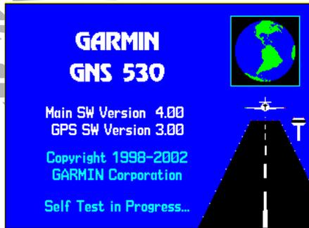
The Welcome Page appears when the GNS 530 is powered on. During the time this screen is displayed, the GNS 530 performs a self test to ensure proper operation.
