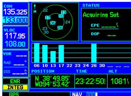
To switch the active and standby frequencies, press the COM flip-flop key. Switching the active and standby frequencies does not remove the cursor from the COM window.
