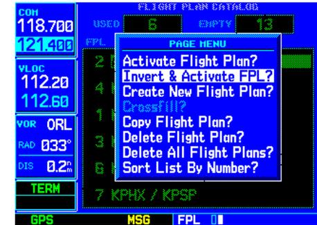
“Activate Flight Plan?” selects the highlighted flight plan and uses it for navigation guidance. “Invert & Activate FPL?” reverses the order of waypoints in the flight plan, then selects it for navigation guidance.
