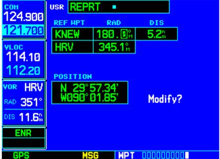
STEP 5: With the radial (RAD) field highlighted, use the **small** and **large right knobs** to enter a new radial from the reference waypoint.
