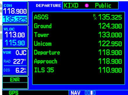
Tuning cursor in the COM window. Use the **small** and **large left knobs** to dial in the desired standby frequency.
