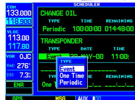
STEP 4 (top): Rotate the **small right knob** to select the desired message type. One Time and Periodic messages appear when the time expires. Event-based messages expire at a specified time and date.
