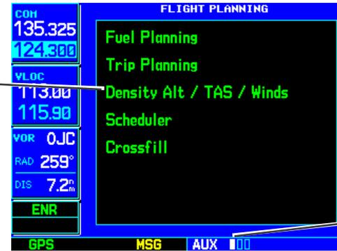
The Flight Planning Page provides access (via a list of “menu options”) to E6B functions for fuel planning, trip planning, density altitude/true airspeed/winds aloft calculations, scheduled messages and a “Crossfill” function to transfer flight plans/user waypoints to a second GNS 530. When a menu option is selected, the corresponding page appears providing additional information and features.
