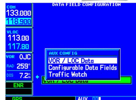
STEP 2: Rotate the **small right knob** to select the desired data field option.
