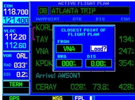
To determine the closest point where the active flight plan passes a particular waypoint, use the "Closest Point of FPL?" option. A waypoint can be added to the flight plan at the calculated location.
