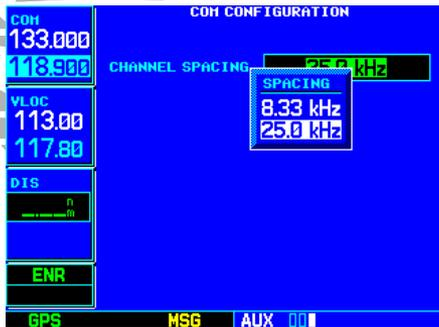
8.33 kHz and 25.0 kHz channel spacing are available for the GNS 530's COM transceiver. Use the 25.0 kHz setting in the United States.
