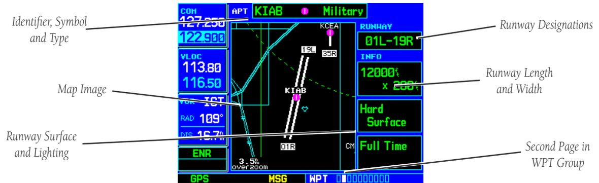
The Airport Runway Page displays runway designations, length, surface type and lighting for the selected airport. A map image of the runway layout and surrounding area is also displayed on the Airport Runway Page. The map image scale appears in the lower left corner and is adjustable using the **RNG** key. For airports with multiple runways, information for each runway is available.
