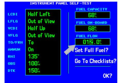
Enter the fuel capacity, fuel on board or fuel flow figures directly onto the appropriate field of the Instrument Panel Self-Test Page. Fuel on board and fuel flow are automatically provided if your installation includes connection to external sensors.
