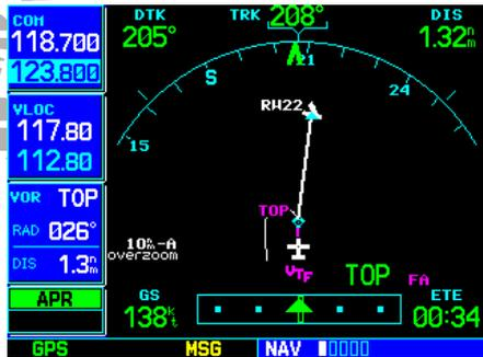
STEP 6: At 2.0 nautical miles from the FAF, the GNS 530 switches from terminal (“TERM”) to approach (“APR”) mode. The CDI scale transitions from 1.0 to 0.3 nautical mile, full scale.
