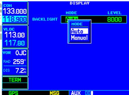
STEP 2 (top): Rotate the **small right knob** to select the backlight mode. If "Manual" is selected, use the **small right knob** to select the backlight level.
