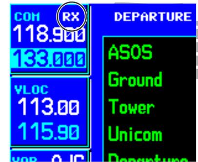
Press the **COM power/volume knob** momentarily to override the automatic squelch. Note the "RX" receive indication when receiving a station.
