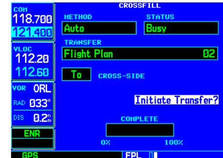
Once “Initiate Transfer?” is selected, a progress bar at the bottom of the page indicates the status of the crossfill transfer until completed.
