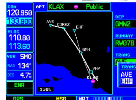
STEP 7: With the "TRANS" field highlighted, rotate the **small right knob** to select the desired transition.
