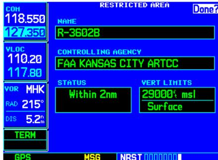
STEP 3 & 4: From the Nearest Airspace Page, highlight the desired airspace and press **ENT** to display additional airspace information.
