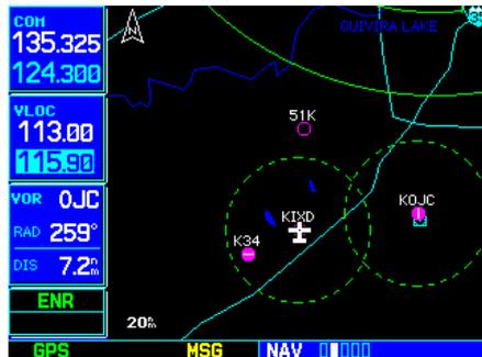
Step 3: To activate the standby frequency, press the **VLOC flip-flop** key.
