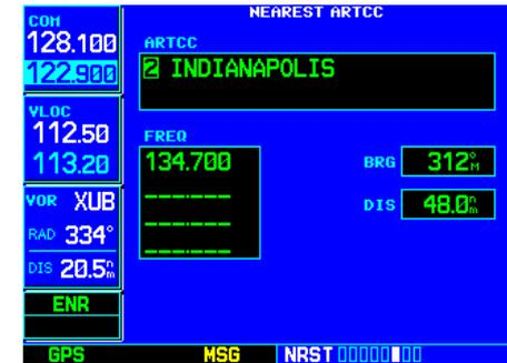
To scroll through the ARTCC or FSS frequencies, highlight the number adjacent to the communication point name and rotate the **small right knob**.
