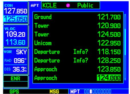
Rotate the **large right knob** to scroll through the list.
