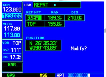
STEP 3 & 4: Use the **small** and **large right knobs** to enter the name of the reference waypoint. Press **ENT** and the cursor moves to the radial (RAD) field.
