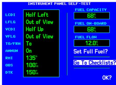
Select “Go To Checklists?” to display the Checklist Page and any available checklists. The GNS 530 can hold up to nine checklists with up to 30 entries in each checklist.
