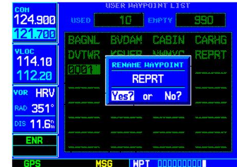
STEP 3 & 4 (bottom): From the User Waypoint List, use the **small and large right knobs** to rename an existing waypoint. Press **ENT** to display a "Rename Waypoint" confirmation window.
