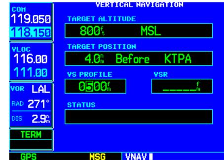
STEP 8: The default profile is a 400 foot-per-minute climb/descent. Use the **small** and **large right knobs** to enter a different vertical speed figure.
