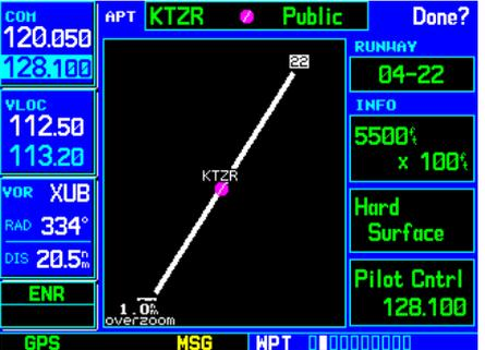
STEP 5: To display additional database information, press the **small right knob** to remove the cursor, then rotate the **small right knob** to select the desired page.
