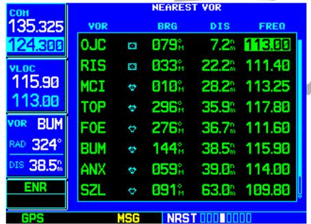
STEP 3 & 4 (top): To automatically tune a VLOC frequency, highlight the desired frequency on the VOR or Nearest VOR Pages, and press **ENT**.
