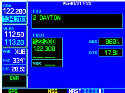
STEP 5 & 6 (next page): Press **ENT** to place the frequency on standby. Press the **COM** or **VLOC flip-flop** key to activate the selected frequency. Navigation frequencies for ILS and localizer (LOC) also appear on the list.
