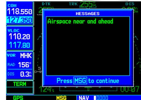
“*Airspace near and ahead*” indicates that you are within two nautical miles of an airspace and projected to enter the airspace.
