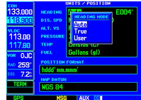
STEP 2 (top): Rotate the **small right knob** to select the desired heading mode. The default setting is "Auto", which automatically calculates the magnetic variation at your current position.
