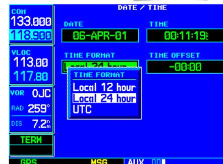
STEP 2 & 3 (top): Rotate the **small right knob** to select the desired time format.
