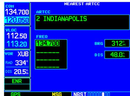
STEP 5 & 6: Press **ENT** to place the frequency in standby. Press the **COM flip-flop** key to activate the selected frequency.
