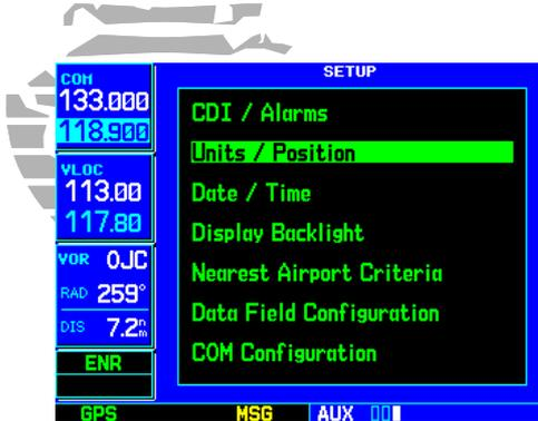
STEP 2: From the Setup Page, highlight the desired menu option and press **ENT**...
