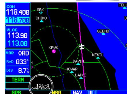
To quickly declutter the map, press **CLR**. Continue pressing **CLR** to select the desired declutter level. Note the scale is followed “-1”, “-2” or “-3”.
