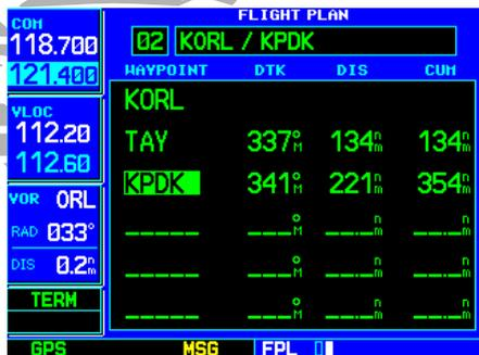
Highlight the point in the existing flight plan where you wish to add the new waypoint. If an existing waypoint is highlighted, the new waypoint is placed directly in front of it.
