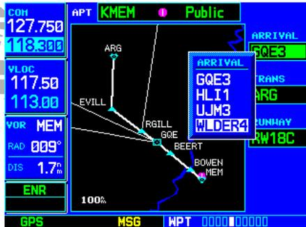
STEP 2 & 3: With the cursor on the “ARRIVAL” field, rotate the **small right knob** to display a list of available arrival procedures.
