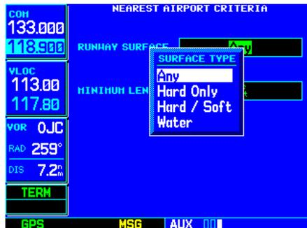
STEP 2 (bottom): Use the **small right knob** to select the desired runway surface type. Select "Any" to include all runway surface types.
