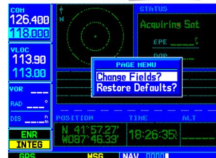
By default, current altitude (ALT) is displayed in the lower right corner of the page. This field is user selectable using the "Change Fields?" option.
