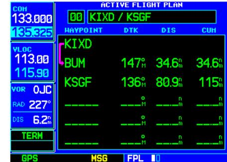
Active Flight Plan Page with flight plan currently in use.
