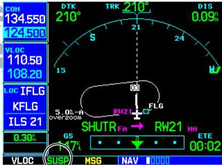
“SUSP” indicates that automatic sequencing of approach waypoints is suspended. In some instances “SUSP” automatically cancels (holding pattern entry). In other cases, press **OBS** to manually cancel
