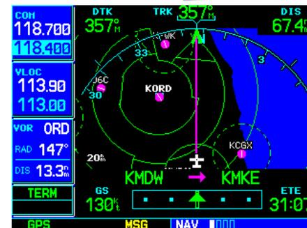
Nine map scale settings are available on the Default NAV Page — from 5.0 to 200 nautical miles. To adjust the map scale, use the **RNG** key.
