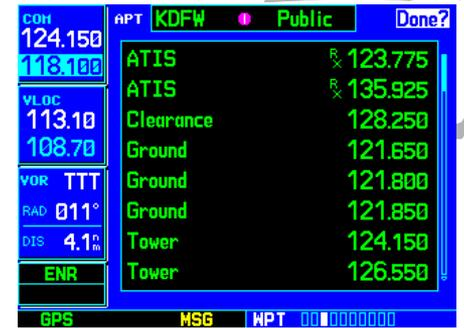
STEP 2: Highlight “View Frequencies?” and press **ENT** to display the communication frequency(s) for the controlling agency.
