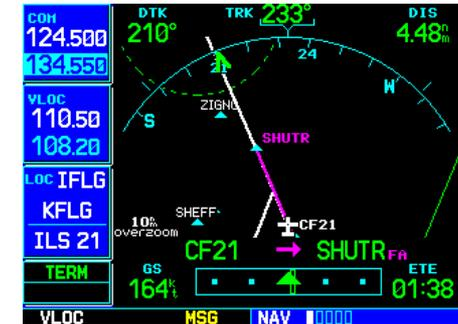
Within the shaded area of the illustration at left, the GNS 530 automatically switches the external CDI to the GNS 530's internal VLOC receiver. "VLOC" appears above the **CDI** key.
