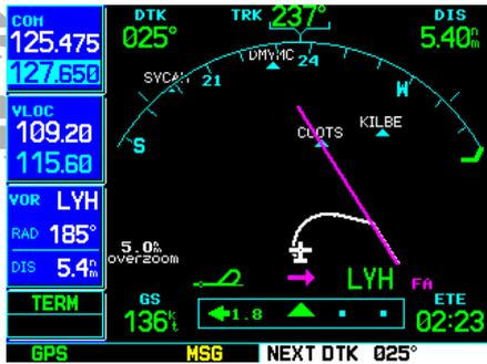
STEP 7 & 8: Procedure turn, inbound. The CDI needle swings to the opposite side for proper sensing and “NEXT DTK 025°” appears. Turn to the new heading as the needle begins to center.
